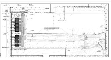
will be a new street (Loren Drive) constructed along the south side of the subject lot in the future, a public sidewalk will also be required along the south lot line, but this can be installed when this street is constructed in the future. This future public sidewalk has been noted on the site plan. Private sidewalk connections to the townhomes will also be provided as shown. **Criterion met.**
